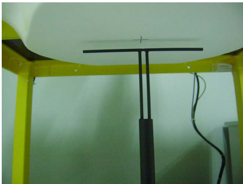
Setup Photo of Dipole Antenna
