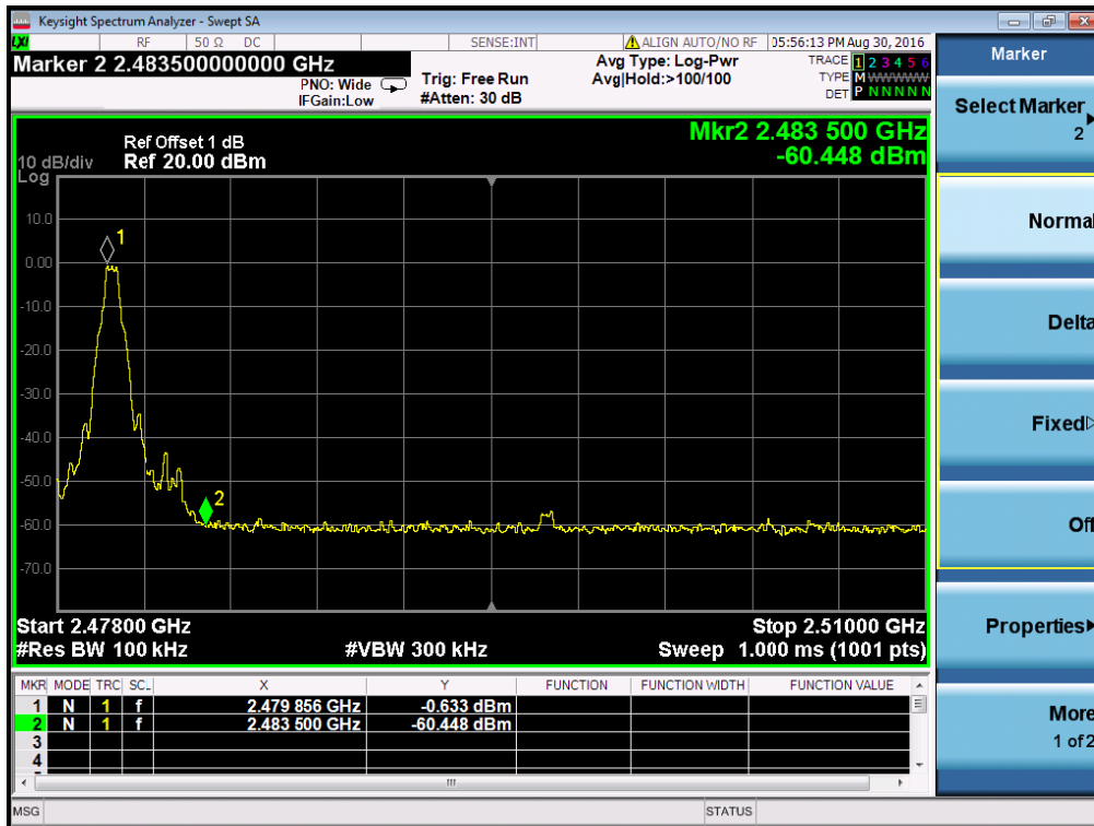
High Band Edge Plot on channel 78 @ GFSK
