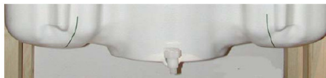
Figure 7.2 SAM Twin Phantom shell
