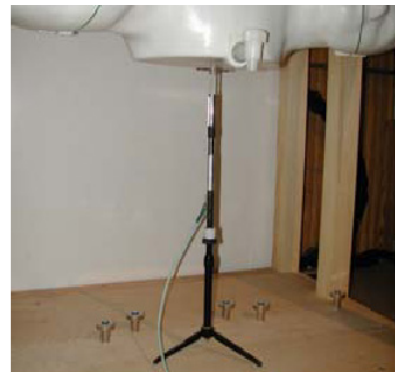
Figure 12.1 Dipole Validation Test Setup
