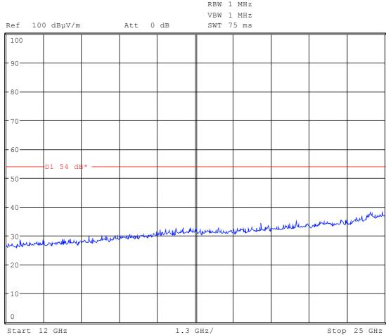
For this measurement we used a special wideband horn antenna and a low noise preamp.
