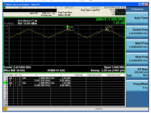
Carrier Frequency Separation (AFH) Hopping mode: Enable & Test Case 1
