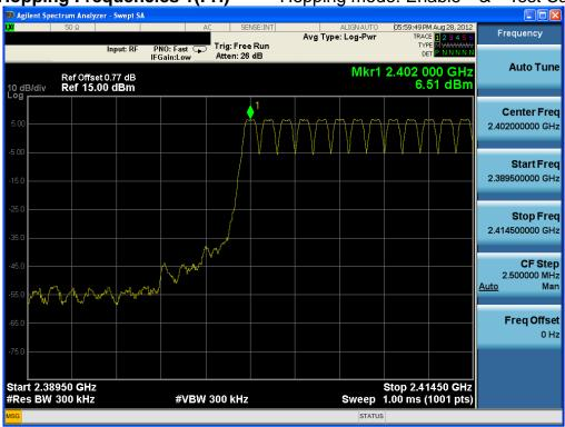
Number of Hopping Frequencies 2(FH) Hopping mode: Enable & Test Case 1
