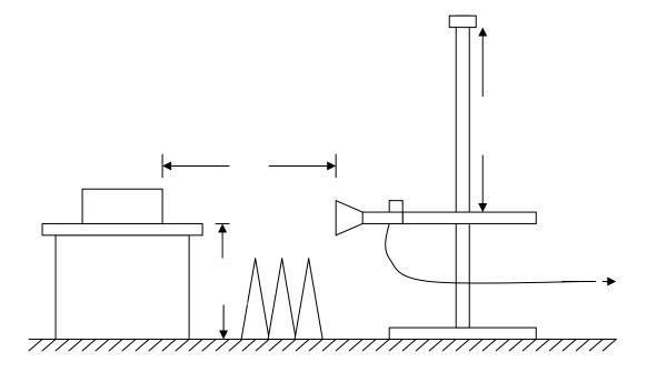
Frequency :9kHz-30MHz RBW=10KHz, VBW =30KHz Sweep time= Auto Trace = max hold Detector function = peak Frequency :30MHz-1GHz RBW=120KHz, VBW=300KHz Sweep time= Auto Trace = max hold Detector function = peak, QP Frequency :Above 1GHz RBW=1MHz, VBW=3MHz(Peak), 10Hz(AV) Sweep time= Auto Trace = max hold Detector function = peak, AV
