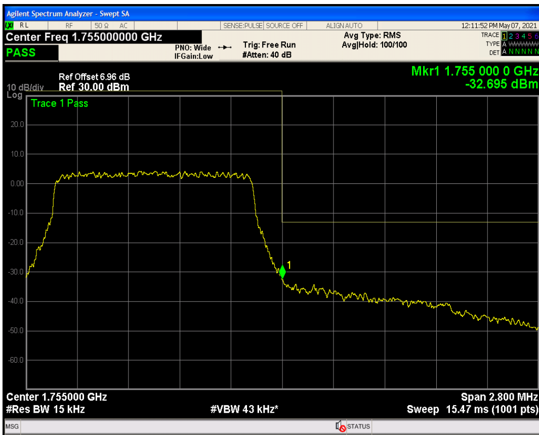
Band4 QPSK BW=3MHz Channel=19965 RB Size=15 Position=#0
