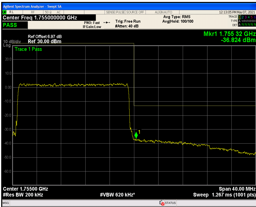
Band41a QPSK BW=5MHz Channel=40265 RB Size=25 Position=#0
