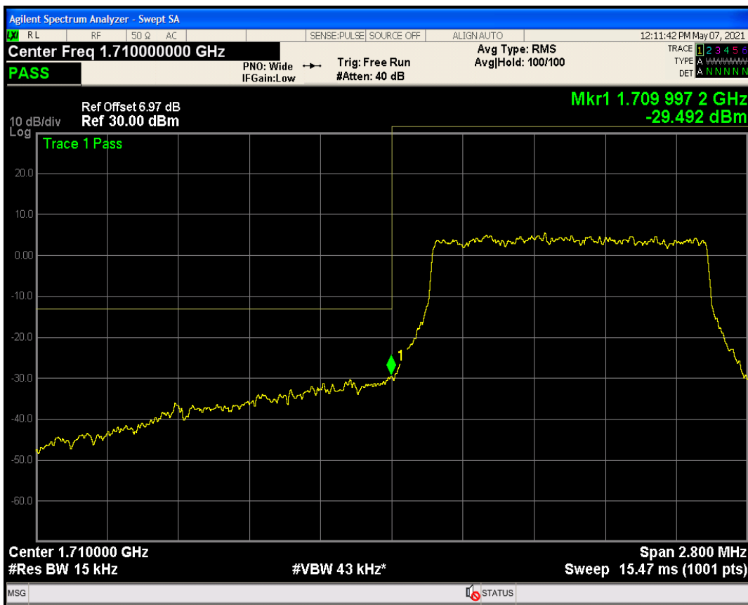
Band4 QPSK BW=1.4MHz Channel=20393 RB Size=6 Position=#0
