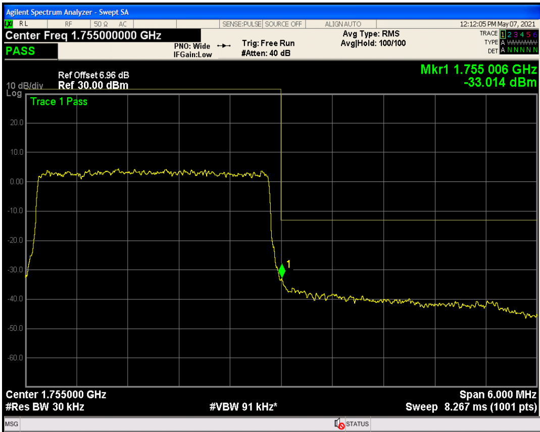
Band4 QAM16 BW=3MHz Channel=20385 RB Size=15 Position=#0
