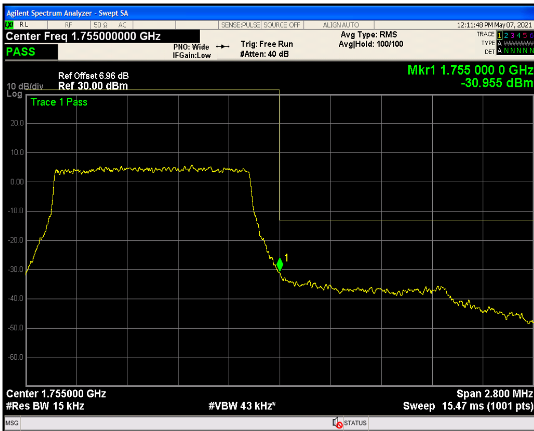
Band4 QAM16 BW=1.4MHz Channel=20393 RB Size=6 Position=#0
