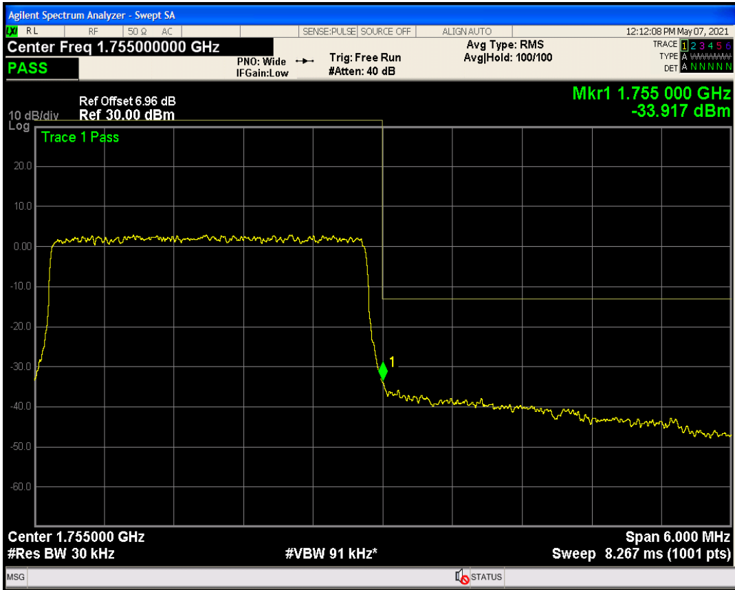
Band4 QPSK BW=5MHz Channel=19975 RB Size=25 Position=#0
