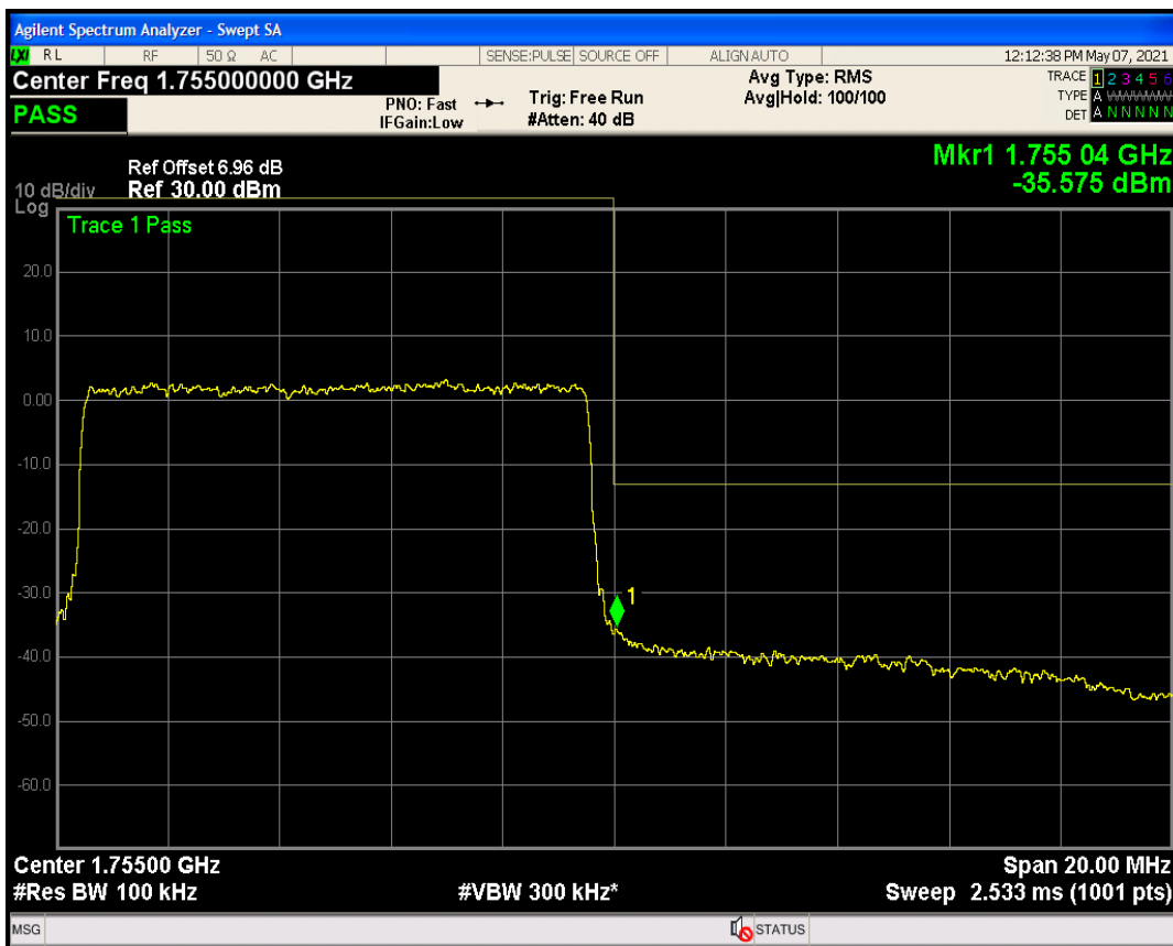
Band4 QPSK BW=15MHz Channel=20025 RB Size=75 Position=#0
