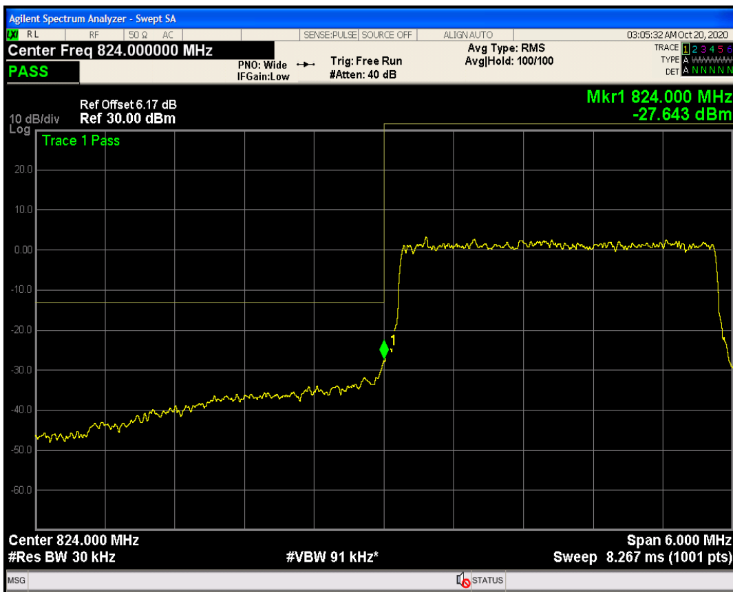
Band5 QPSK BW=3MHz Channel=20635 RB Size=15 Position=#0
