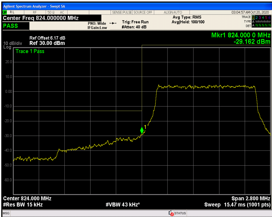
Band5 QAM16 BW=1.4MHz Channel=20407 RB Size=6 Position=#0
