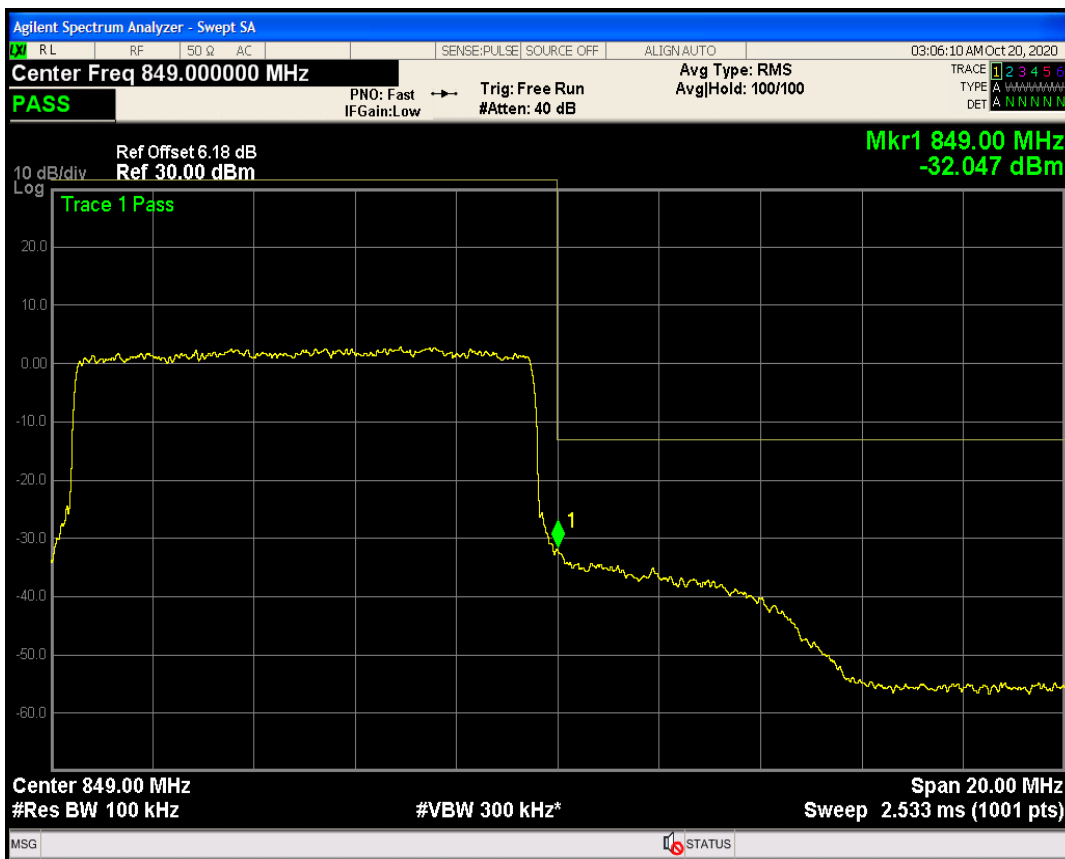
Band7 QPSK BW=5MHz Channel=20775 RB Size=25 Position=#0
