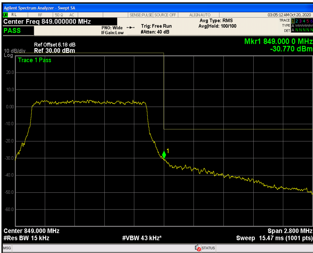
Band5 QPSK BW=3MHz Channel=20415 RB Size=15 Position=#0
