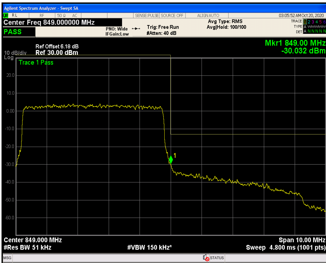
Band5 QAM16 BW=5MHz Channel=20625 RB Size=25 Position=#0
