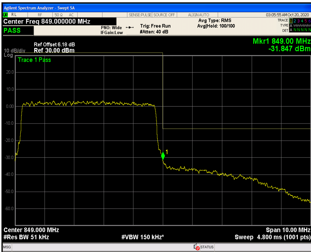
Band5 QPSK BW=10MHz Channel=20450 RB Size=50 Position=#0
