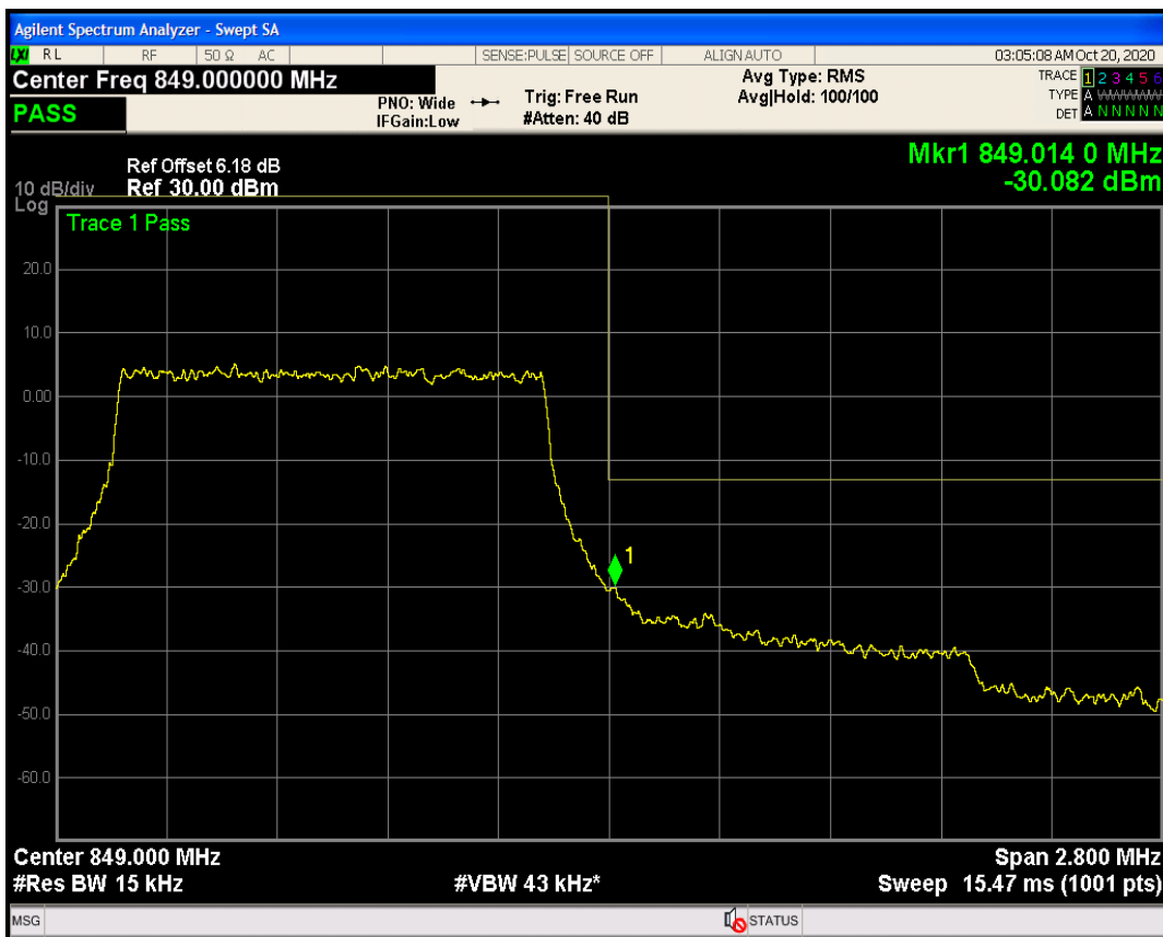
Band5 QAM16 BW=1.4MHz Channel=20643 RB Size=6 Position=#0
