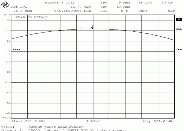
Comment A: CZ600, subtest 1 HSUPA FDD V, output power, channel 4233 (846.6MHz)
