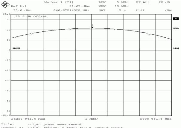
Comment A: CZ600, subtest 4 HSUPA FDD V, output power, channel 4233 (846.6MHz)
