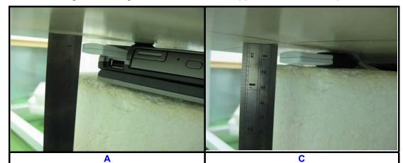
The bottom of the EUT faces to the phantom with The front of the EUT faces to the phantom with 5mm-separation distance.
