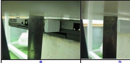
The right edge of the EUT faces to the phantom with 5mm-separation distance.
