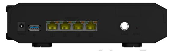
**Important:** Do not connect your PC to both the Ethernet and USB ports at the same time. Your residential gateway will not function properly if both the Ethernet and USB ports are connected to your PC at the same time.
