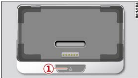
Fig. 21 Rear centre armrest/centre console extending into rear cabin: Holder for Rear Seat Remote
