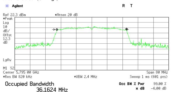
Transmit Freq Error -464.980 Hz x dB Bandwidth 34.372 MHz
