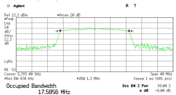
Transmit Freq Error -22.438 kHz x dB Bandwidth 17.261 MHz
