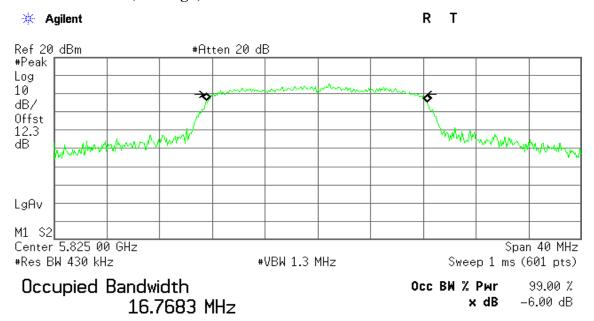
Transmit Freq Error -79.922 kHz x dB Bandwidth 15.578 MHz
