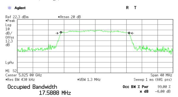
Transmit Freq Error -36.688 kHz x dB Bandwidth 17.446 MHz
