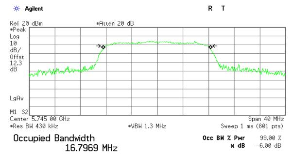
Transmit Freq Error -94.065 kHz x dB Bandwidth 16.100 MHz
