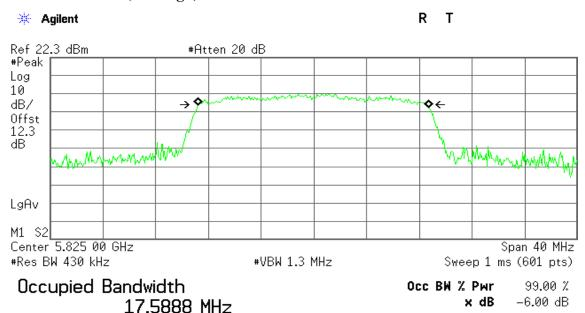
Transmit Freq Error -36.688 kHz x dB Bandwidth 17.446 MHz
