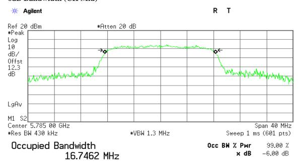
Transmit Freq Error -18.464 kHz x dB Bandwidth 15.976 MHz
