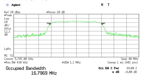
Transmit Freq Error -94.065 kHz x dB Bandwidth 16.100 MHz
