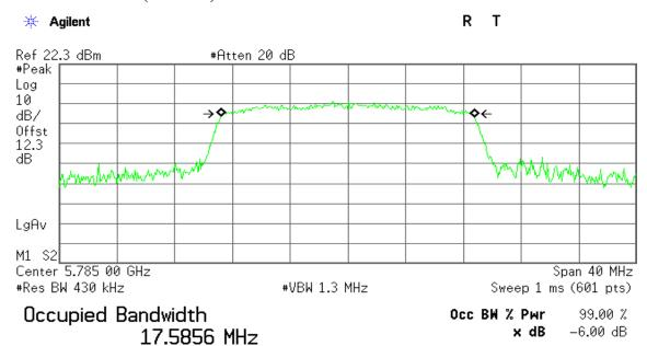
Transmit Freq Error -22.438 kHz x dB Bandwidth 17.261 MHz
