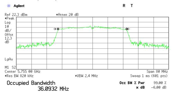
Transmit Freq Error -42.967 kHz x dB Bandwidth 34.862 MHz
