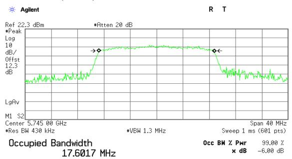
Transmit Freq Error -11.833 kHz x dB Bandwidth 17.242 MHz
