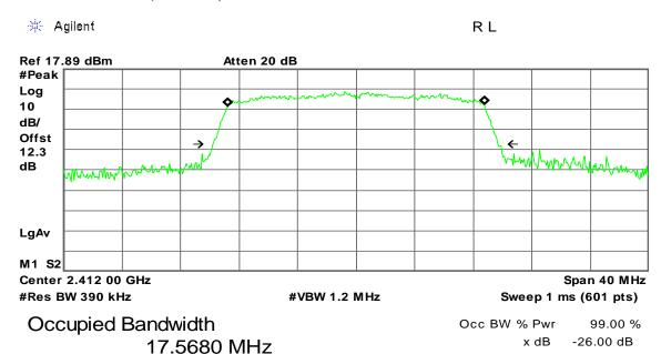
Transmit Freq Error -9.108 kHz x dB Bandwidth 19.511 MHz
