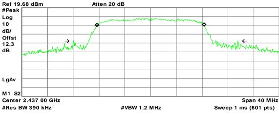
Occupied Bandwidth 16.6772 MHz Occ BW % Pwr 99.00 % x dB -26.00 dB
