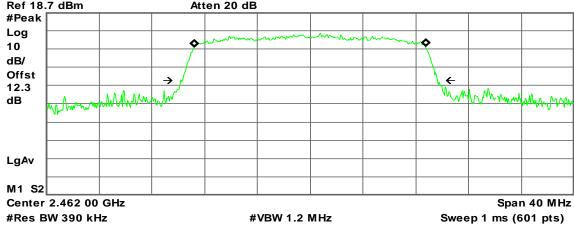
Occupied Bandwidth 17.5702 MHz Occ BW % Pwr 99.00 % x dB -26.00 dB
