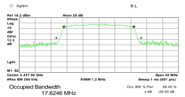
Transmit Freq Error -9.211 kHz x dB Bandwidth 19.519 MHz
