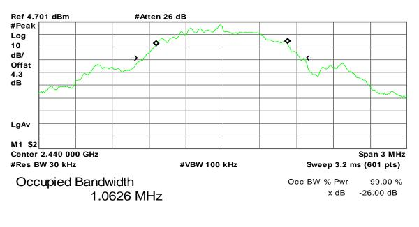
Transmit Freq Error-7.445 kHzx dB Bandwidth1.273 MHz
