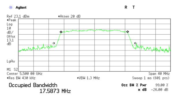
Transmit Freq Error -29.168 kHz x dB Bandwidth 19.524 MHz
