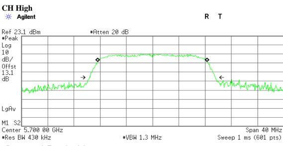
Occupied Bandwidth 16.6956 MHz Occ BW % Pwr 99.00 % x dB -26.00 dB
