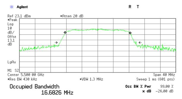
Transmit Freq Error 12.316 kHz x dB Bandwidth 19.517 MHz
