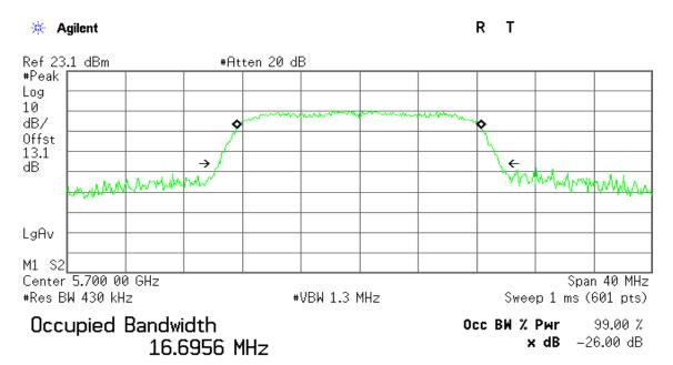
Transmit Freq Error -24.278 kHz x dB Bandwidth 19.158 MHz
