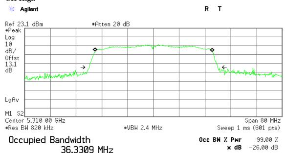
Transmit Freq Error 64.352 kHz x dB Bandwidth 39.916 MHz
