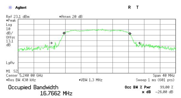
Transmit Freq Error 17.299 kHz x dB Bandwidth 20.570 MHz
