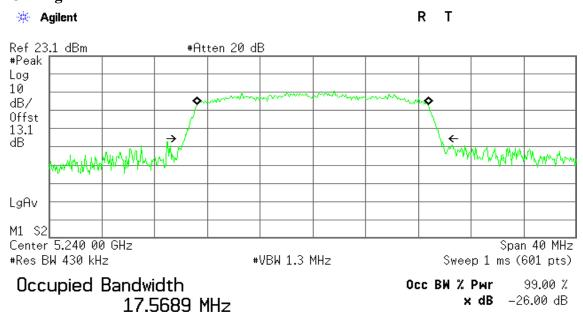
Transmit Freq Error -16.486 kHz x dB Bandwidth 19.378 MHz
