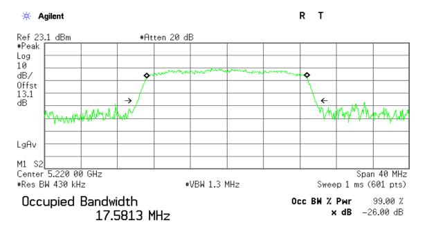
Transmit Freq Error -23.397 kHz x dB Bandwidth 19.494 MHz
