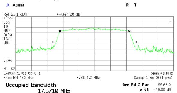
Transmit Freq Error -42.988 kHz x dB Bandwidth 19.502 MHz
