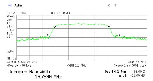
Transmit Freq Error 14.003 kHz x dB Bandwidth 20.344 MHz
