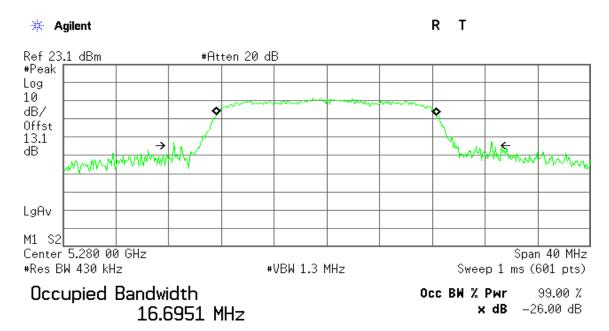
Transmit Freq Error -21.889 kHz x dB Bandwidth 24.186 MHz
