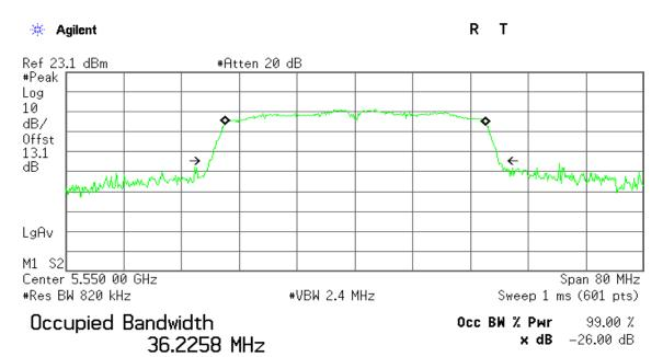
Transmit Freq Error 65.709 kHz x dB Bandwidth 40.046 MHz
