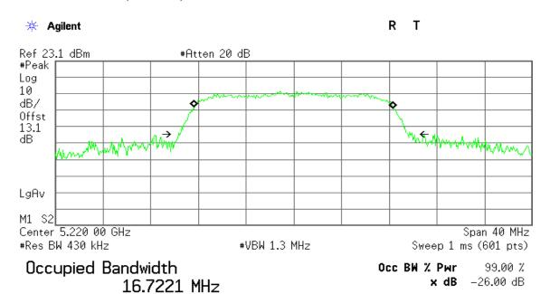
Transmit Freq Error -6.033 kHz x dB Bandwidth 19.637 MHz
