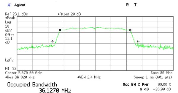
Transmit Freq Error 8.798 Hz x dB Bandwidth 40.017 MHz
