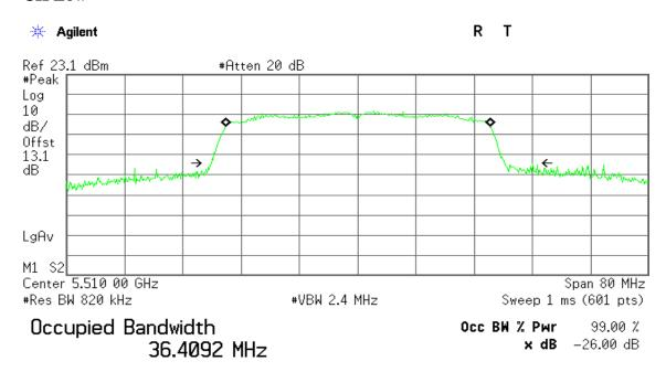
Transmit Freq Error 51.391 kHz x dB Bandwidth 44.121 MHz
