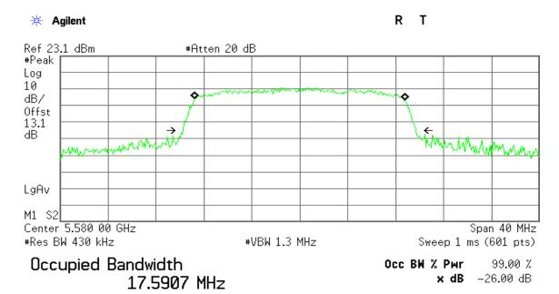
Transmit Freq Error -22.254 kHz x dB Bandwidth 19.495 MHz
