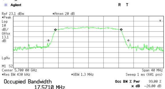
Transmit Freq Error -42.988 kHz x dB Bandwidth 19.502 MHz
