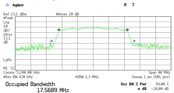
Transmit Freq Error -16.486 kHz x dB Bandwidth 19.378 MHz
