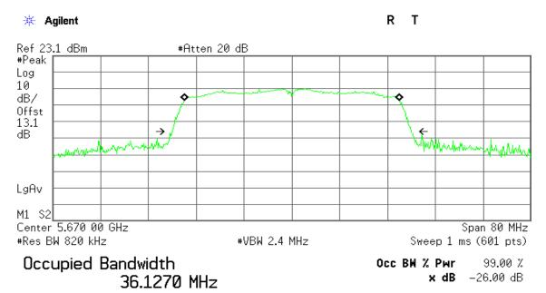
Transmit Freq Error 8.798 Hz x dB Bandwidth 40.017 MHz
