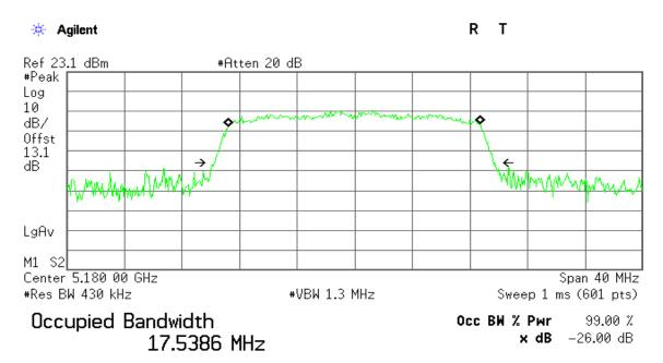
Transmit Freq Error -27.433 kHz x dB Bandwidth 19.360 MHz
