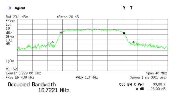
Transmit Freq Error -6.033 kHz x dB Bandwidth 19.637 MHz
