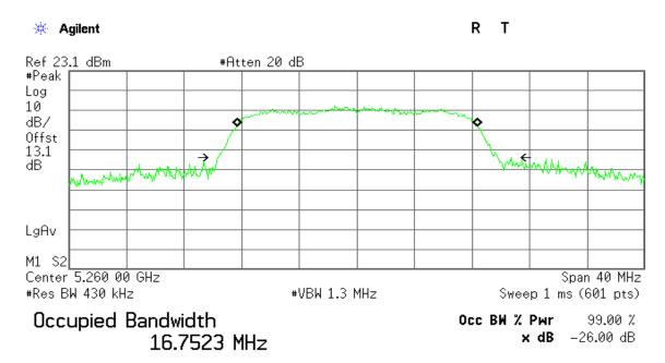
Transmit Freq Error 28.519 kHz x dB Bandwidth 20.397 MHz
