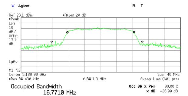
Transmit Freq Error -5.148 kHz x dB Bandwidth 20.825 MHz
