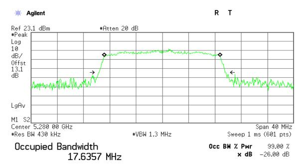
Transmit Freq Error -30.667 kHz x dB Bandwidth 19.334 MHz
