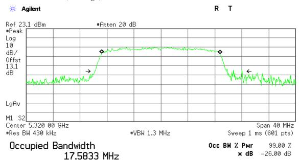
Transmit Freq Error -15.871 kHz x dB Bandwidth 21.854 MHz
