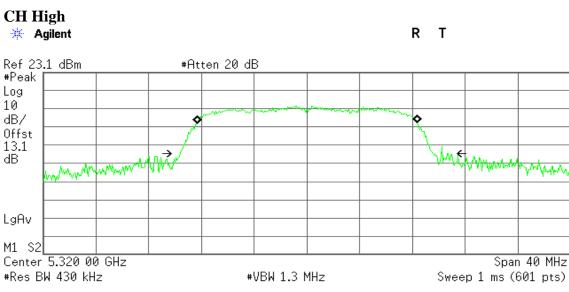
Occupied Bandwidth 16.7580 MHz Occ BW % Pwr 99.00 % x dB -26.00 dB
