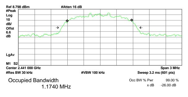
Transmit Freq Error x dB Bandwidth -12.788 kHz 1.383 MHz
