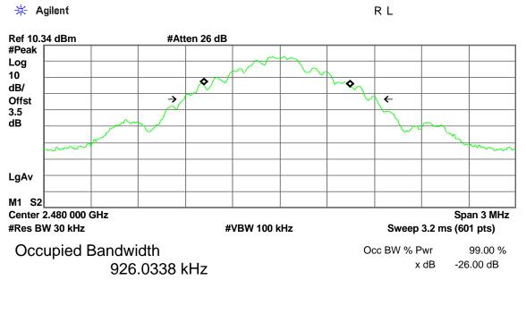
Transmit Freq Error-16.338 kHzx dB Bandwidth1.224 MHz
