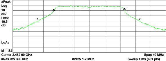
Occupied Bandwidth 18.4920 MHz Occ BW % Pwr 99.00 % x dB -26.00 dB
