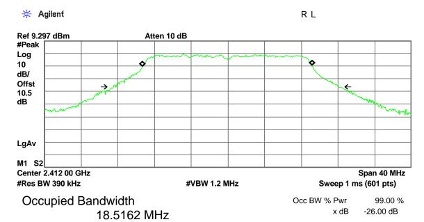
Transmit Freq Error -76.821 kHz x dB Bandwidth 24.513 MHz
