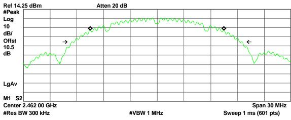
Occupied Bandwidth 14.9896 MHz Occ BW % Pwr 99.00 % x dB -26.00 dB
