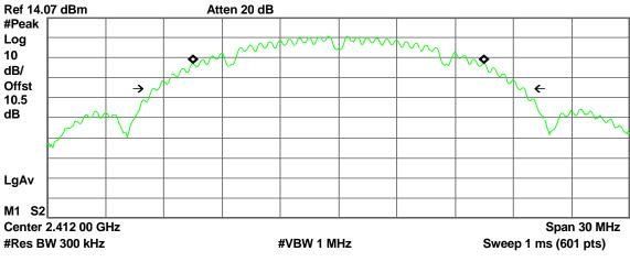
Occupied Bandwidth 14.9847 MHz Occ BW % Pwr 99.00 % x dB -26.00 dB
