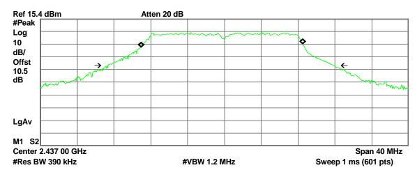
Occupied Bandwidth 17.6216 MHz Occ BW % Pwr 99.00 % x dB -26.00 dB
