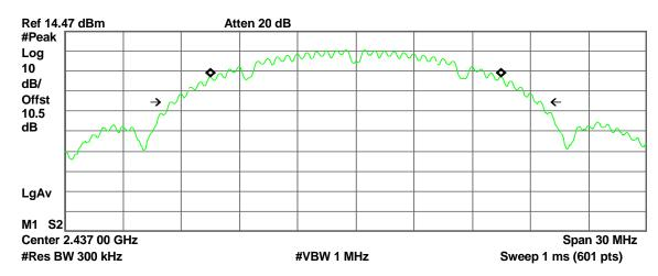
Occupied Bandwidth 14.9923 MHz Occ BW % Pwr 99.00 % x dB -26.00 dB
