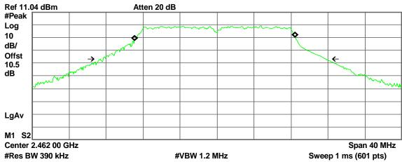
Occupied Bandwidth 17.4479 MHz Occ BW % Pwr 99.00 % x dB -26.00 dB
