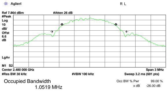
Transmit Freq Error-12.644 kHzx dB Bandwidth1.333 MHz
