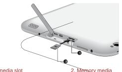
Figure 7-1 Inserting a memory media
