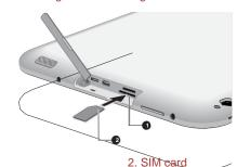
Figure 7-2 Inserting a SIM card
