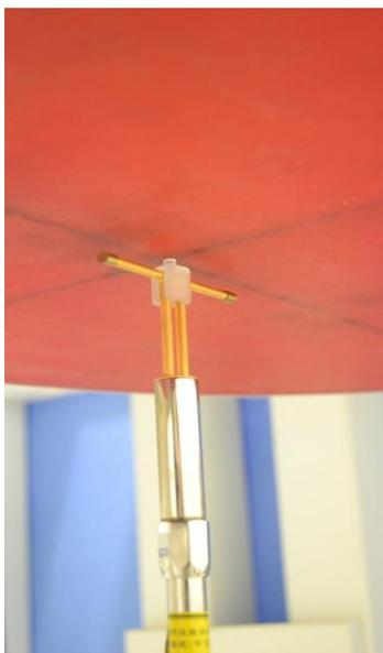
**Construction:** Symmetrical dipole with 1/4 balun Enables measurement of feedpoint impedance with NWA Matched for use near flat phantoms filled with brain simulating solutions Includes distance holder and tripod adaptor.
