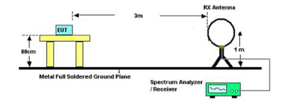
For Radiated Emissions: 30MHz~1GHz
