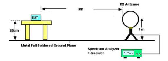
For Radiated Emissions: 30MHz~1GHz
