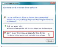
Install the device (if not already installed). When entering Windows for the first time, the device should be detected. Select "**Don't show...**"
