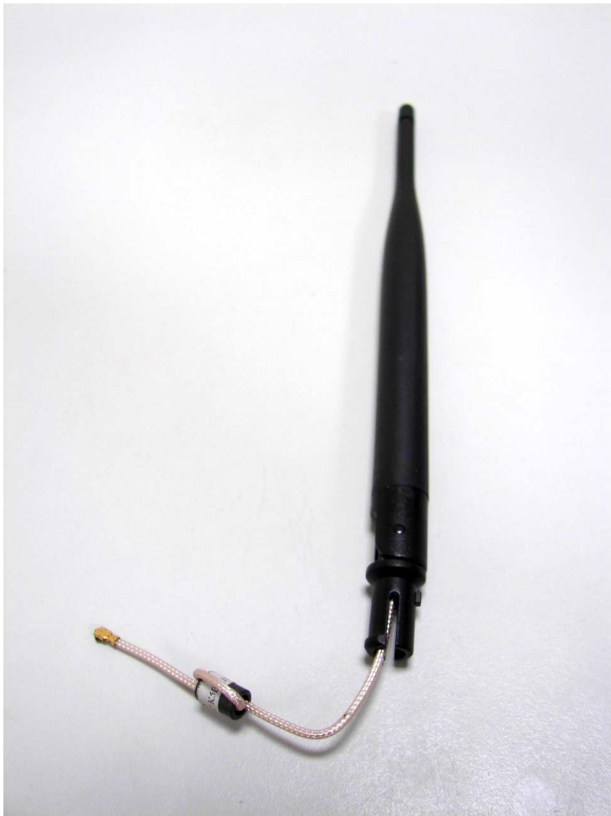
Antenna#1: Dipole antenna
