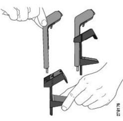
Step 5 With your phone idle (no calls), attach the USB cable to the USB connector on the bottom of the camera.Step 6 Adjust the mounting clip as needed to rest securely on your computer monitor.
