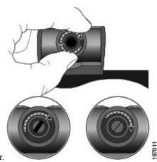
The following figure shows the location of the camera lens shutter.
