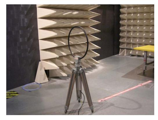
For radiated emissions 30MHz~1GHz
