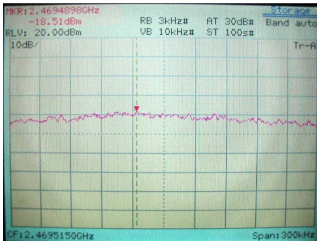
**Power Spectral Density for IEEE 802.11n 20M Channel 01, 2412MHz**
