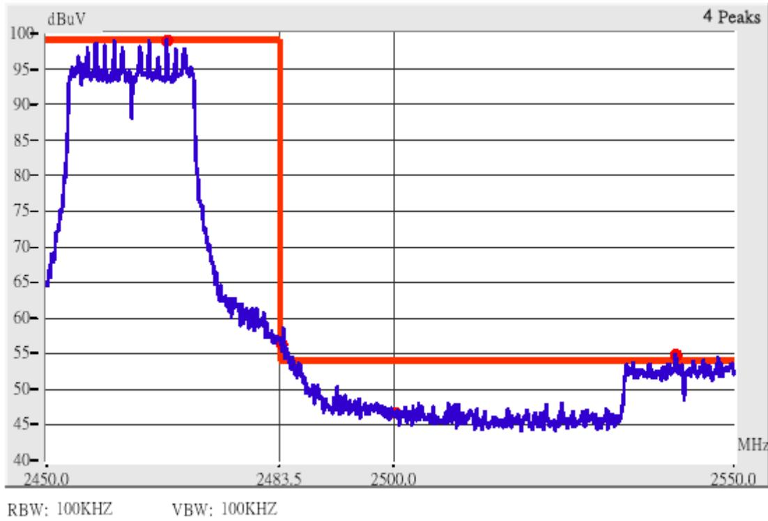
This is the hard copy of our bandedge measurement generated by our bandedge testing program. The plot shown above is the bandedge of channel 11.
