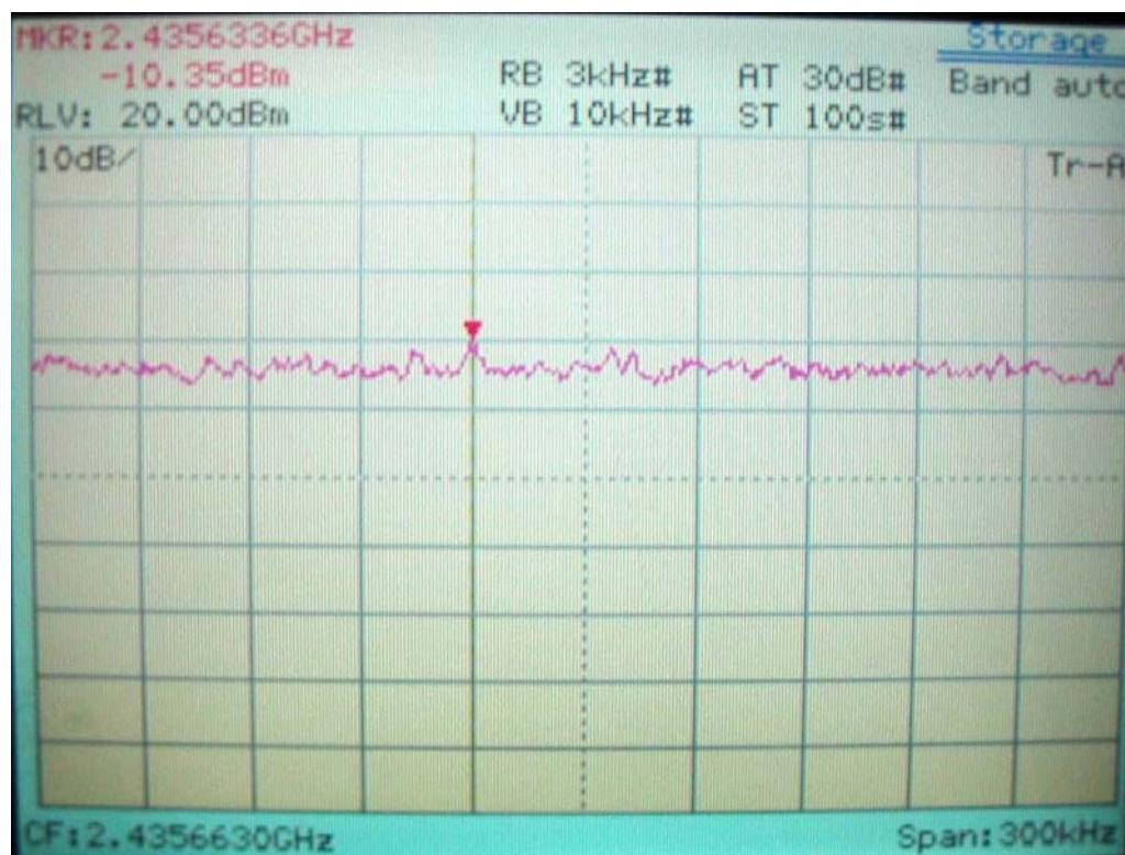
**Power Spectral Density for IEEE 802.11b Channel 11, 2462MHz**
