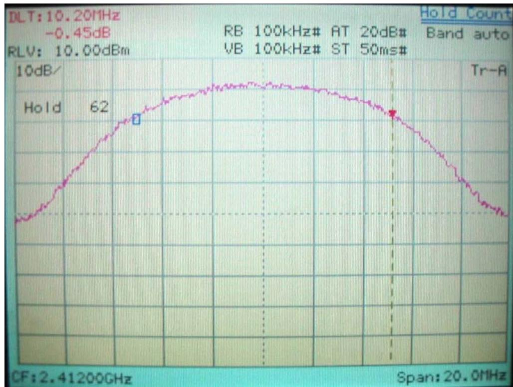
**6dB Bandwidth of Channel CH06 IEEE 802.11b, 2437MHz**
