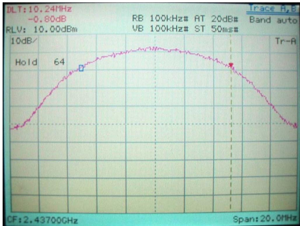
**6dB Bandwidth of Channel CH11 IEEE 802.11b, 2462MHz**
