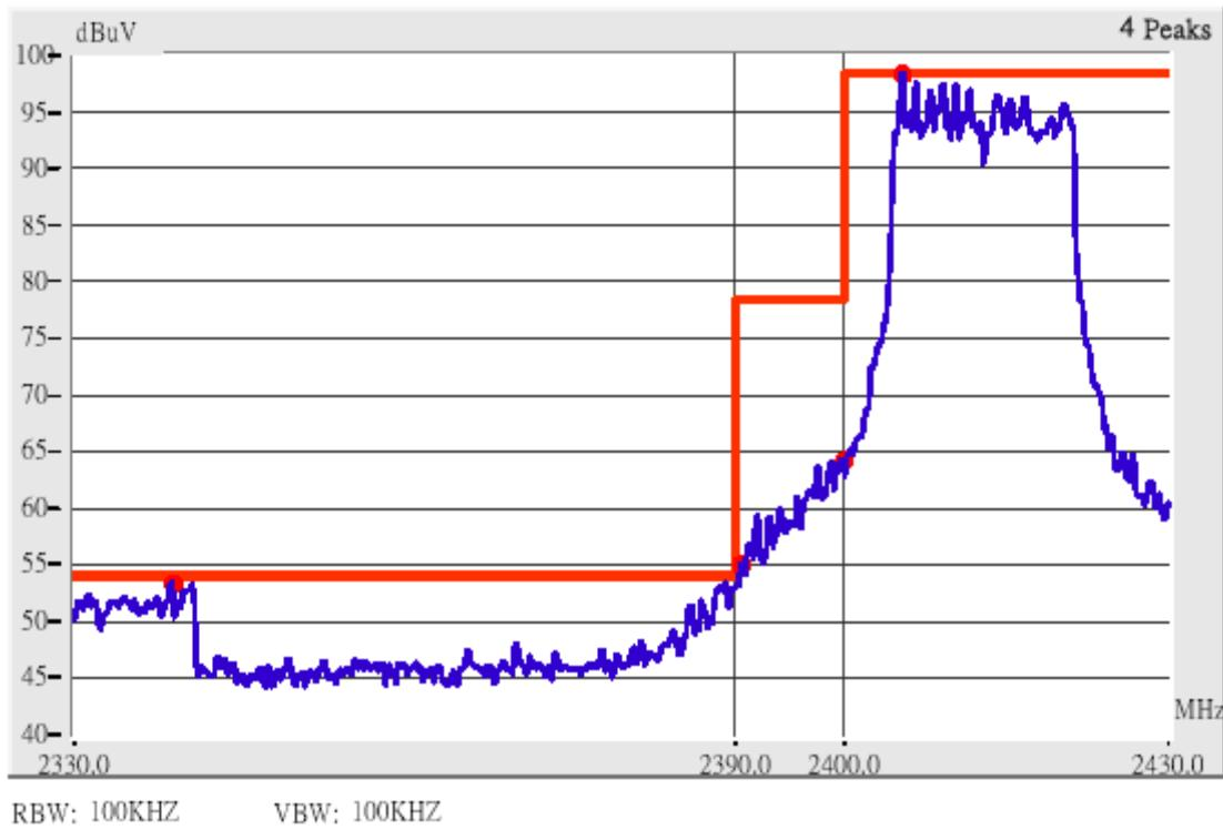
This is the hard copy of our bandedge measurement generated by our bandedge testing program. The plot shown above is the bandedge of channel 1.
