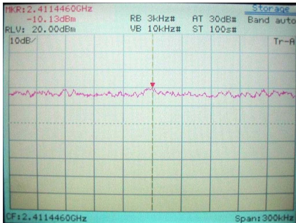
**Power Spectral Density for IEEE 802.11b Channel 06, 2437MHz**
