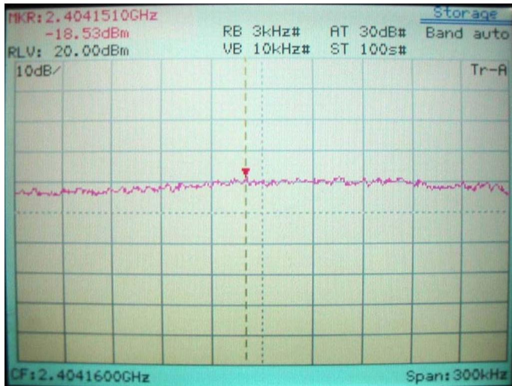
**Power Spectral Density for IEEE 802.11n 20M Channel 06, 2437MHz**
