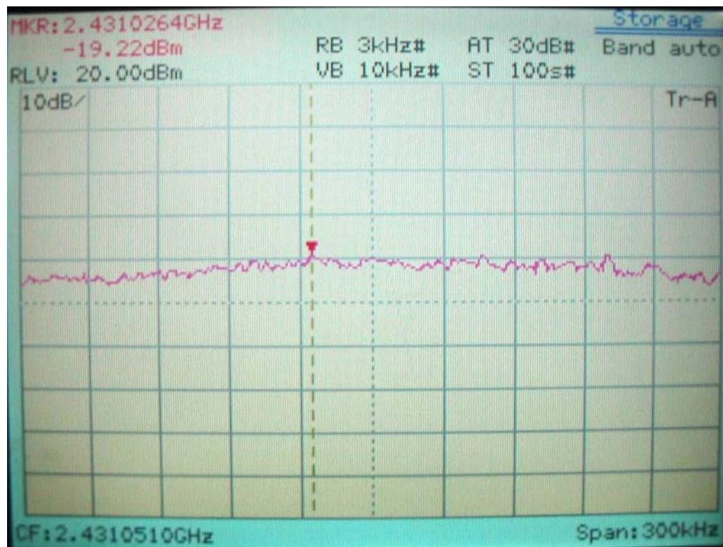
**Power Spectral Density for IEEE 802.11g Channel 11, 2462MHz**
