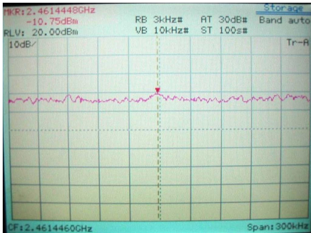
**Power Spectral Density for IEEE 802.11g Channel 01, 2412MHz**
