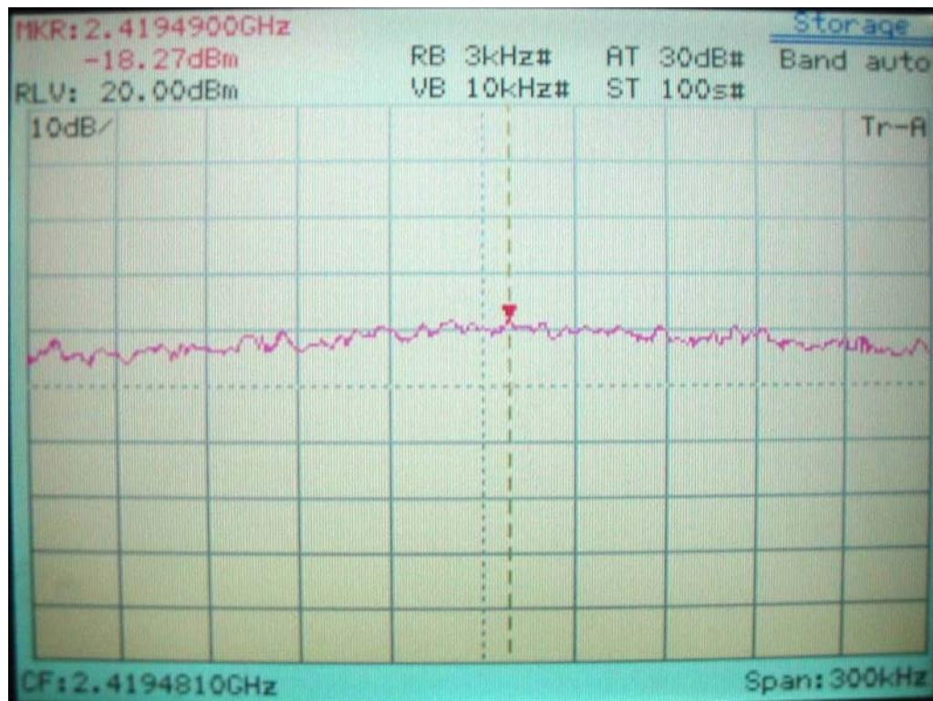
**Power Spectral Density for IEEE 802.11g Channel 06, 2437MHz**
