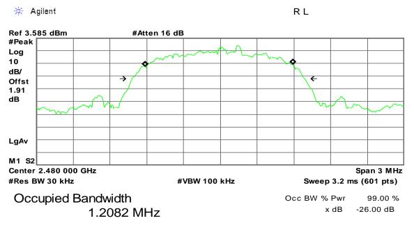
Transmit Freq Error -12.140 kHz x dB Bandwidth 1.410 MHz
