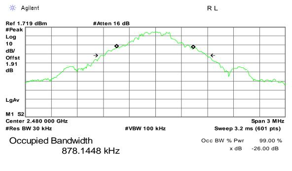
Transmit Freq Error -5.278 kHz x dB Bandwidth 1.200 MHz
