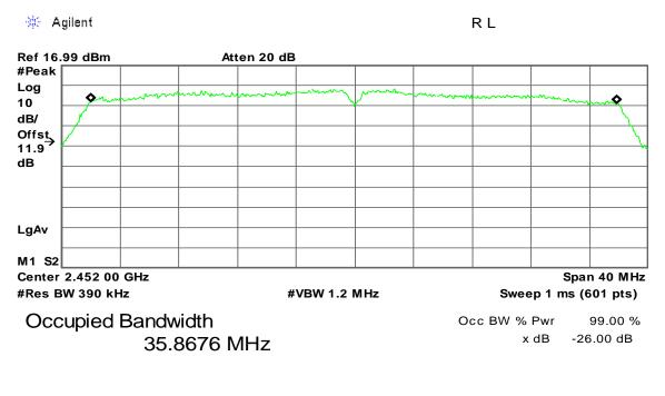
Transmit Freq Error-86.723 kHzx dB Bandwidth39.252 MHz
