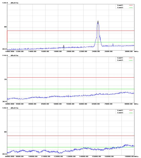
Operation Mode: TX / IEEE 802.11n HT 40 MHz mode / CH Low Test Date: August 9, 2015
