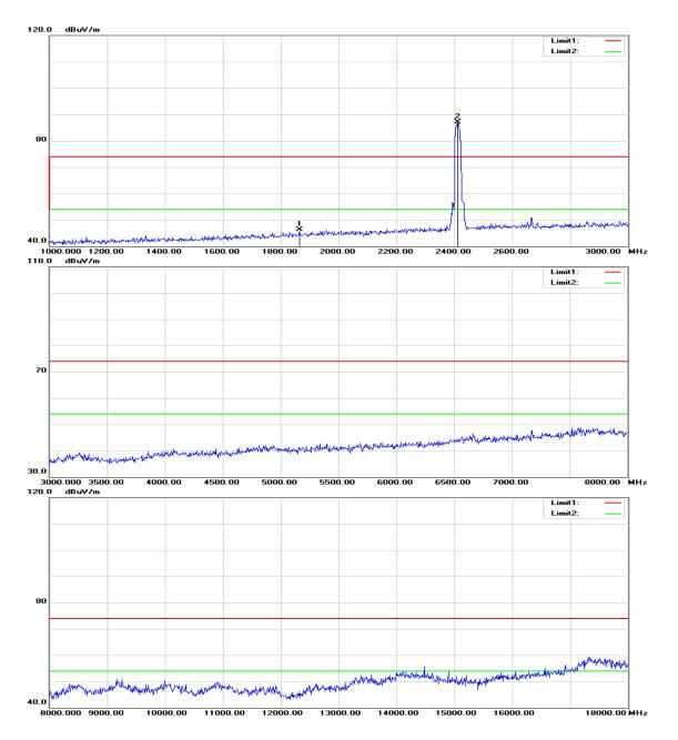
Operation Mode: TX / IEEE 802.11n HT 20 MHz mode / CH Low Test Date: August 9, 2015
