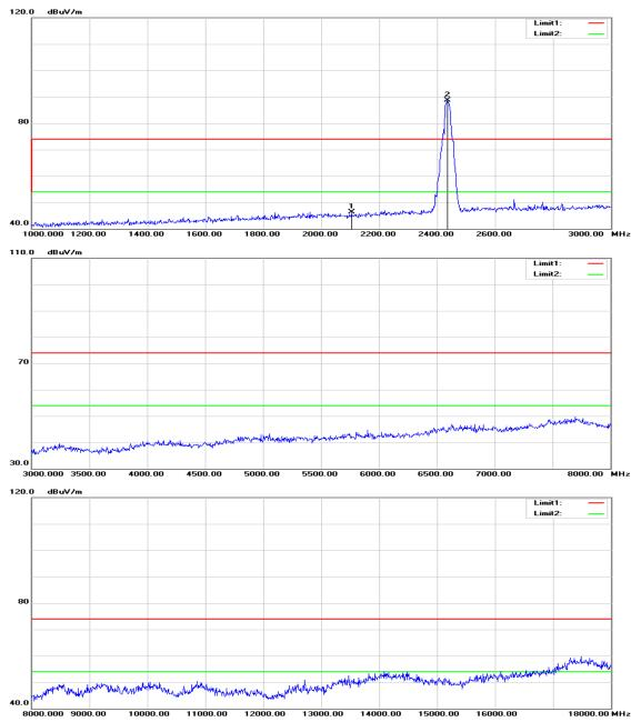
Operation Mode: TX / IEEE 802.11n HT 20 MHz mode / CH Mid Test Date: August 9, 2015
