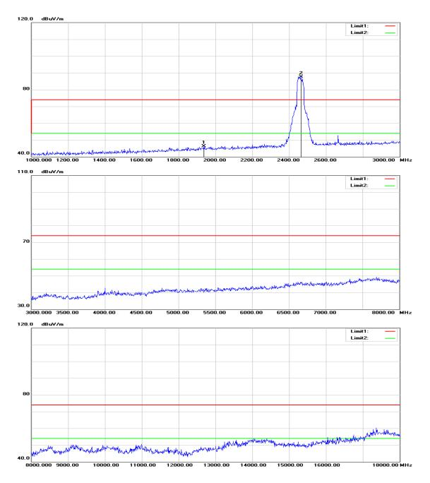
Operation Mode: TX / IEEE 802.11n HT 40 MHz mode / CH High Test Date: August 9, 2015
