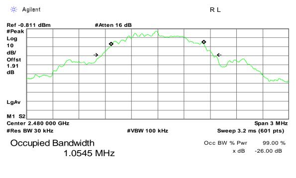
Transmit Freq Error -1.601 kHz x dB Bandwidth 1.269 MHz
