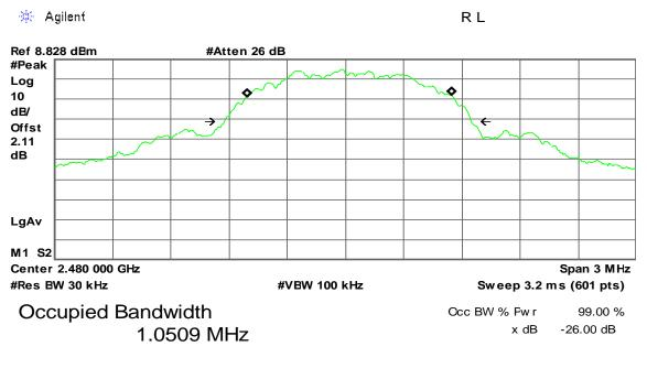
Transmit Freq Error19.656 kHzx dB Bandw idth1.274 MHz
