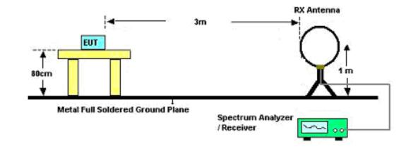
For Radiated Emissions: 30MHz~1GHz
