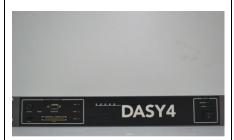
The DASY4/DASY5 measurement server is based on a PC/104 CPU board with a 166MHz low-power Pentium, 32MB chip disk and 64MB RAM. The necessary circuits for communication with either the DAE3 electronic box as well as the 16-bit AD-converter system for optical detection and digital I/O interface are contained on the DASY4/DASY5 I/O-board, which is directly connected to the PC/104 bus of the CPU board.
