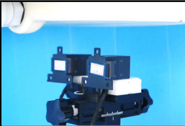
MIMO Front Face of EUT Tested at 41 mm
