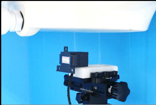
SISO Front Face of EUT Tested at 41 mm
