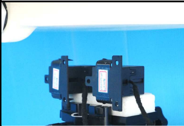
MIMO Right Side of EUT Tested at 41 mm
