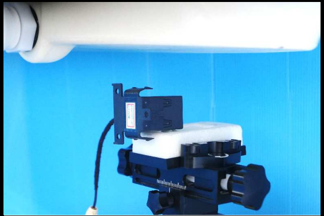
SISO Left Side of EUT Tested at 41 mm
