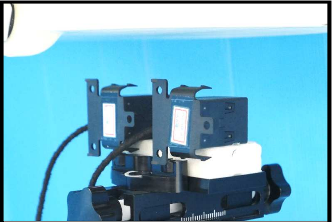
MIMO Left Side of EUT Tested at 41 mm
