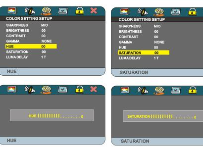
You can set the Hue (for NTSC) to your liking. Press **PLAY/SAVE** or the ► **RIGHT** arrow to enter the Hue control, then press the ▲ UP or ▼ DOWN arrow to adjust the image. Press the ► LEFT arrow to go back to the menu.
