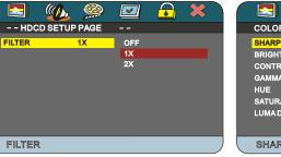
Select HDCD to set up your preferred Audio mode for HDCD. Press **PLAY** to enter this selection and to setup your preferred filter mode for HDCD (default is 1X).
