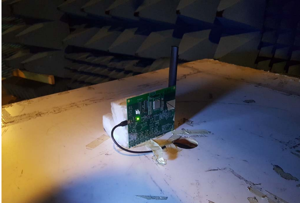
Figure 2 Radiated Emission Test Setup
