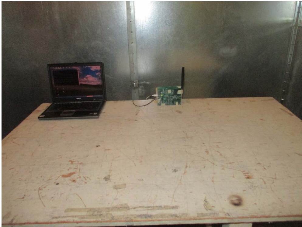
Figure 1 EUT Configuration for Radiated & Conducted Emission Tests
