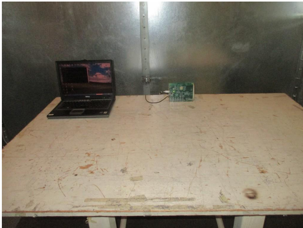
Figure 1 EUT Configuration for Radiated & Conducted Emission Tests
