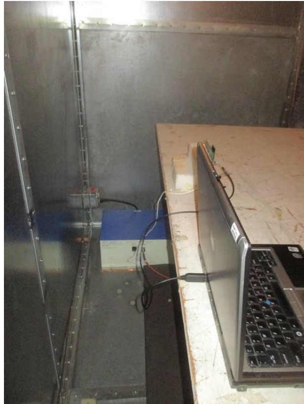
Figure 3 Conducted Emission Test Setup
