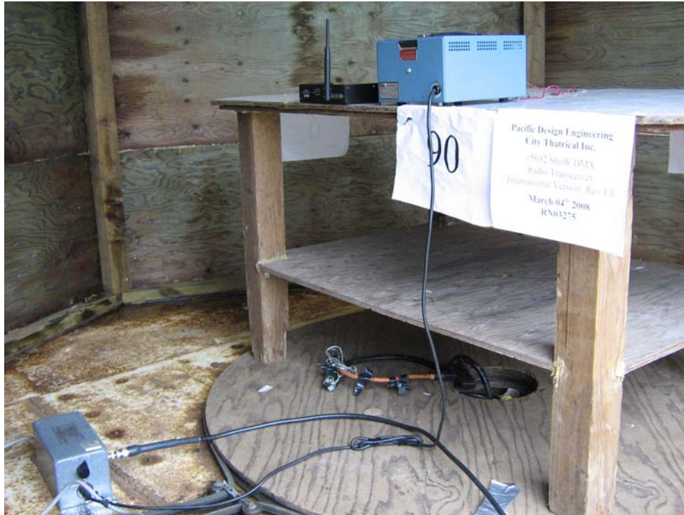
City Theatrical Inc. ShoW DMX Radio Transceiver-# 5692 International Version, AC Conducted Set-up-Figure 4
