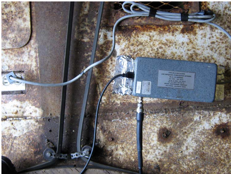
City Theatrical Inc. ShoW DMX Radio Transceiver-# 5692 International Version, AC Conducted Set-up-Figure 4
