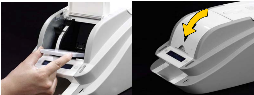
<Figure 17> Placing the cards and close the hopper cover
