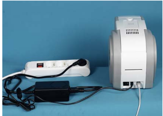
<Figure 18> Connect the power cord
