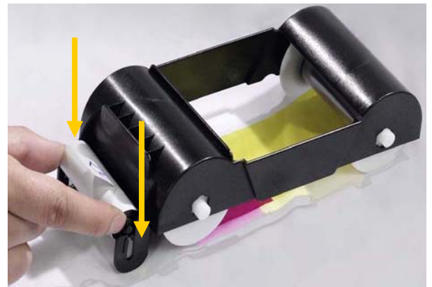
<Figure 9> Install the cleaning roller
