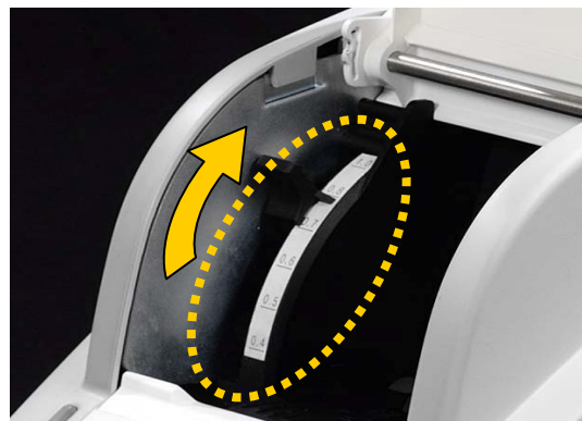
<Figure 13> Adjust the card thickness
