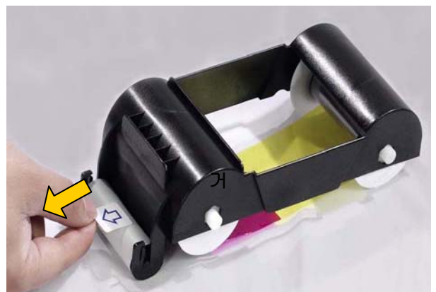
<Figure 10> Peel the protective wrapper
