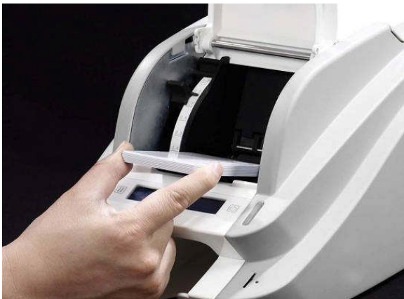
Pic.23 Loading the cards 2
