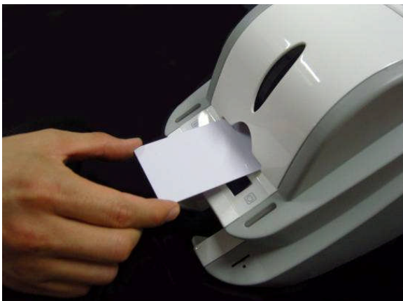
Pic.24 Loading the cards 3
