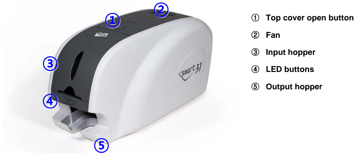
Figure 1 SMART-31 front features
