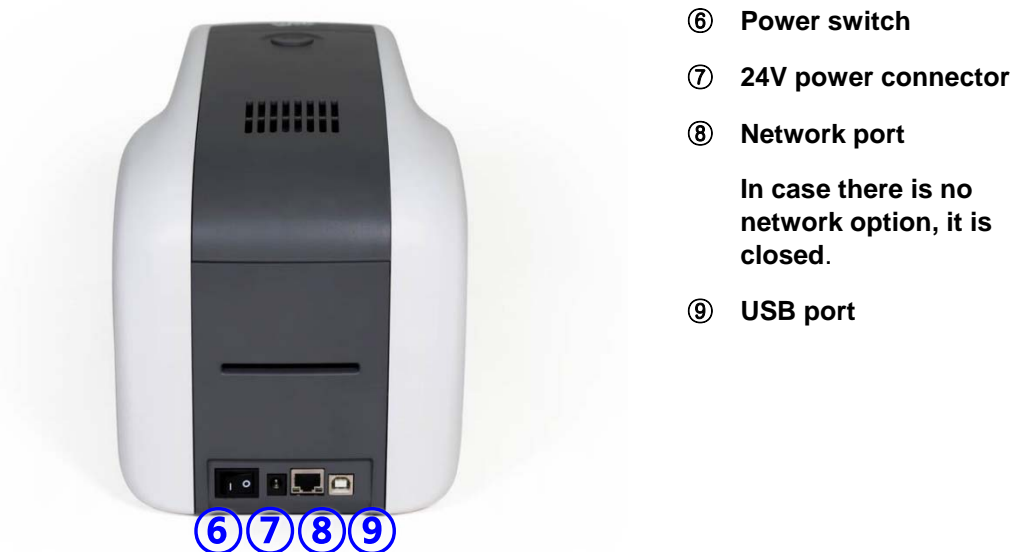
Figure 2 SMART-31 rear features
