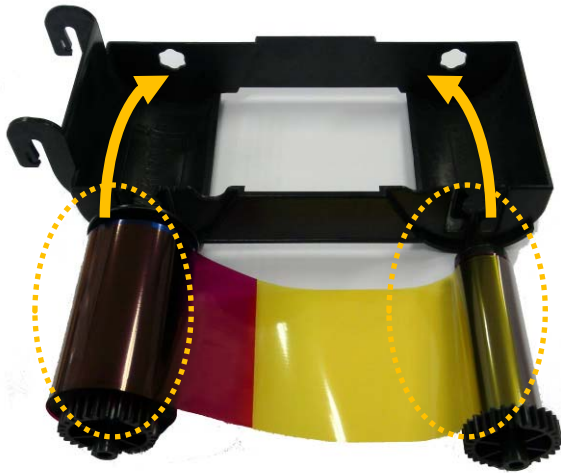
Pic.16 Loading the ribbon 1
