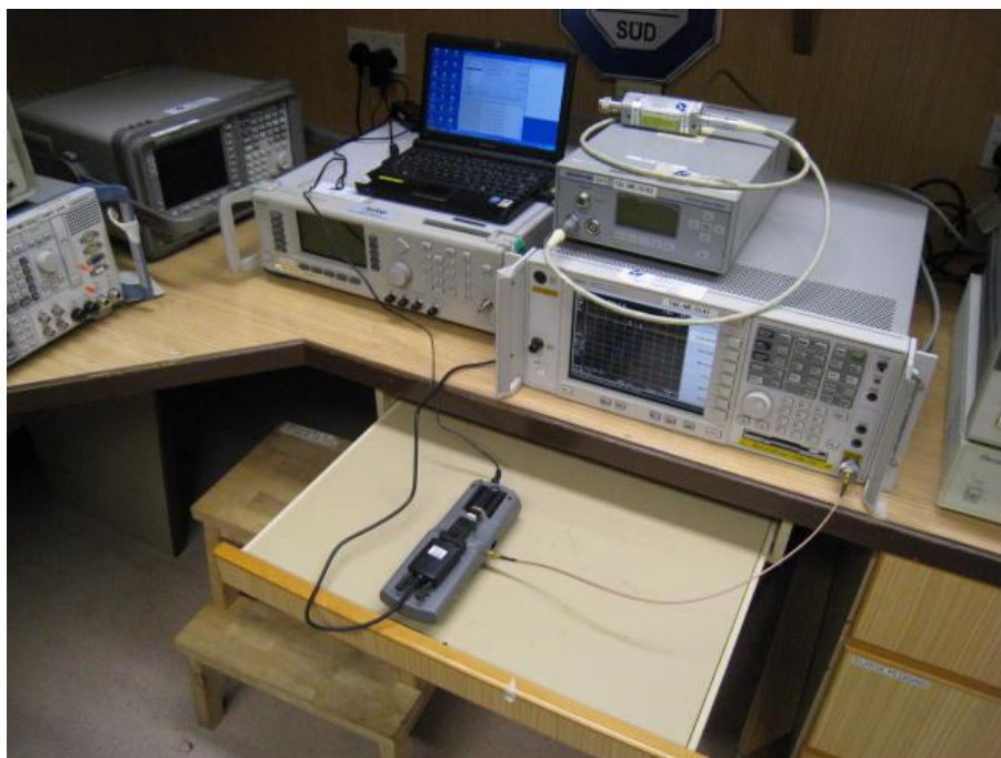
Average Frequency Dwell Time Test Setup
