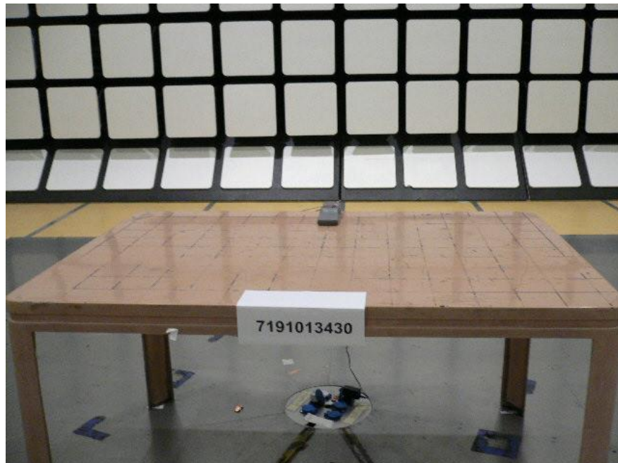
Radiated Emissions Test Setup (Front View)
