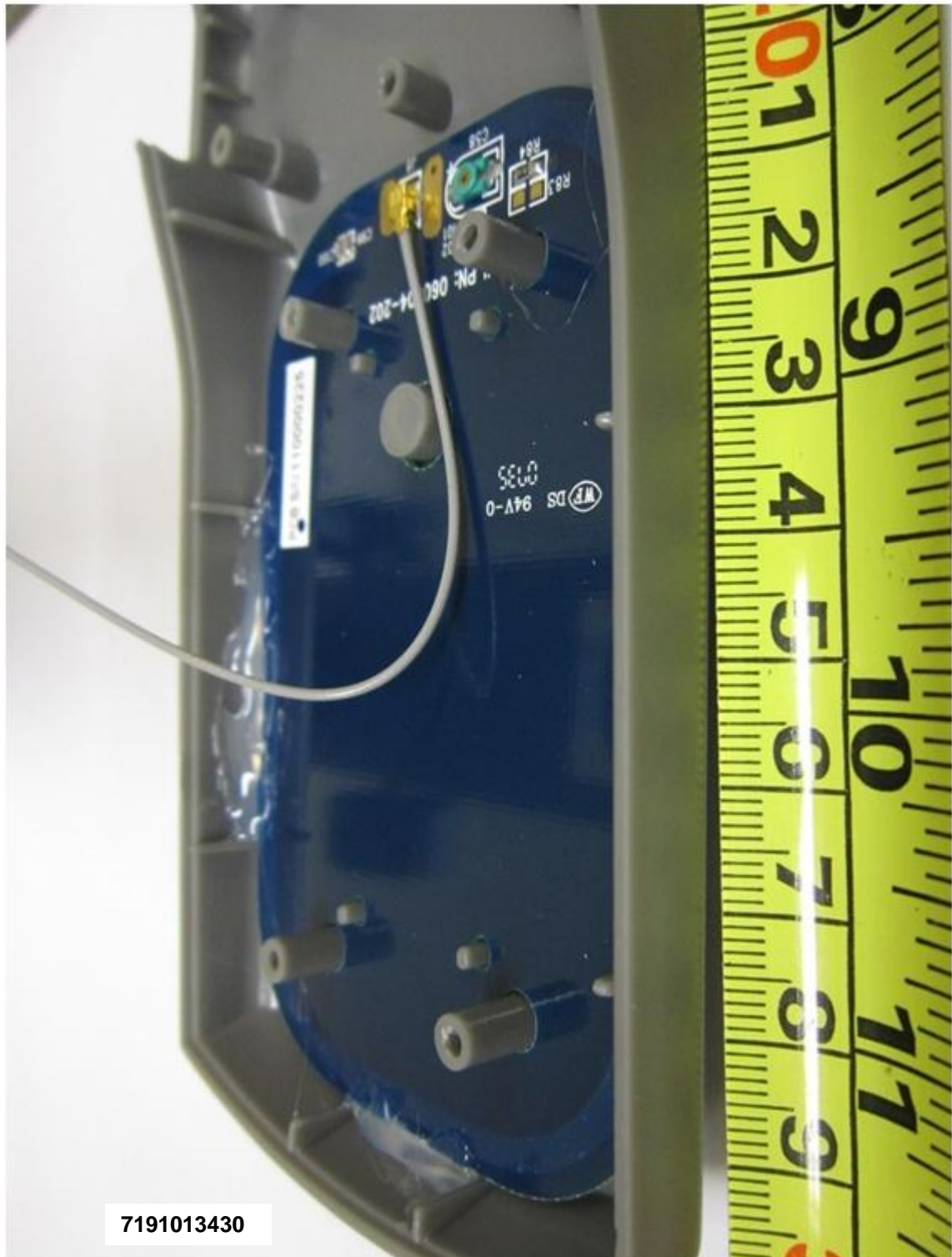
Antenna Board PCB Component Side
