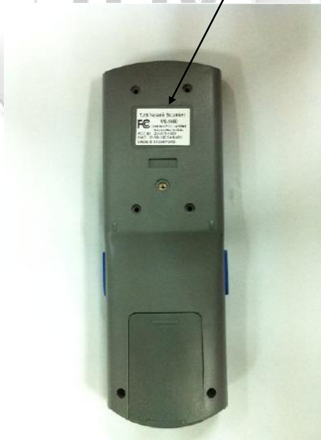
Physical Location of FCC Label on EUT
