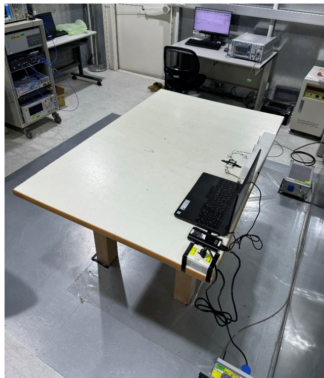
Back View of AC Power Line Conducted Emission Test
