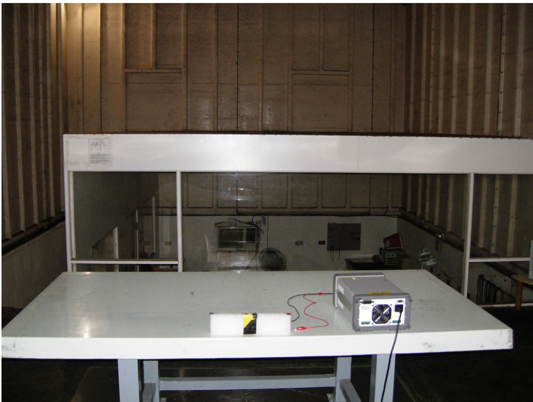
Back View of Radiated Test (below 30MHz) - Loop - Mode 2
