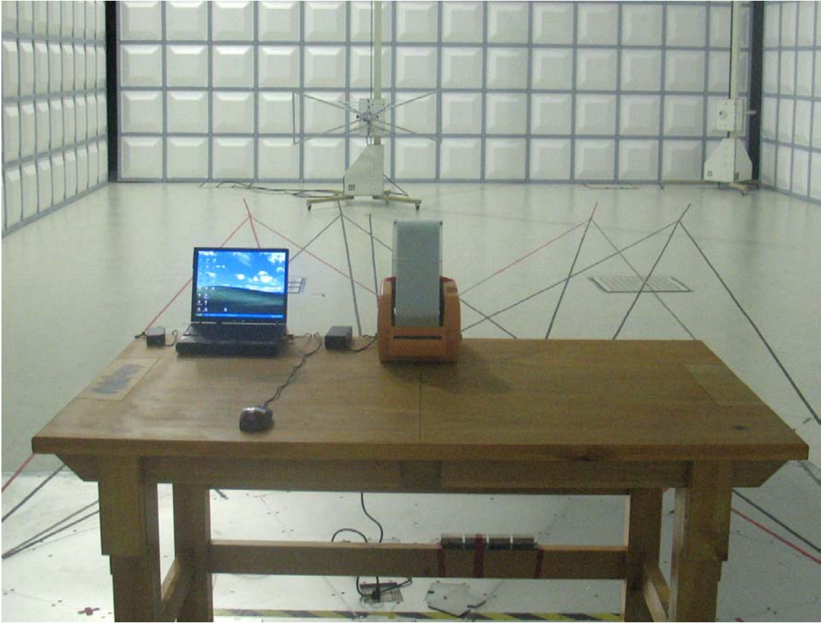
The Back View of Highest Radiated Set-up For EUT
