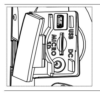
Open the interface cover and connect the printer to the computer with USB cable.
